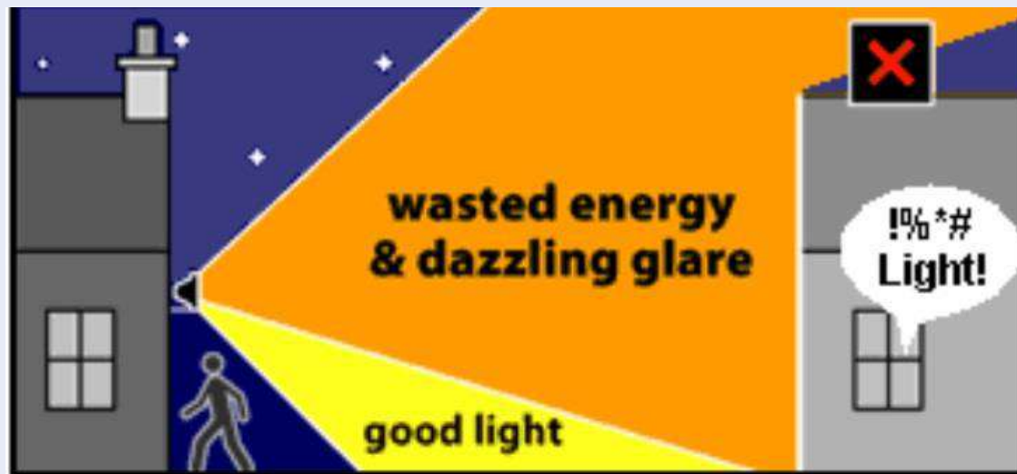
BADLY AIMED 500W HALOGEN FLOODLIGHT
